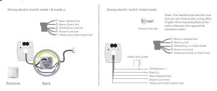
Note: Specific operation see back <Strong electric switch mode selection> action bar.
