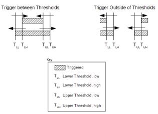
The following diagrams illustrate another way of considering this triggering capability. The X-axis in these diagrams represent time passing (from left to right). The diagrams show the triggering state as the input voltage rises from zero to a certain point and then falls back to zero.
